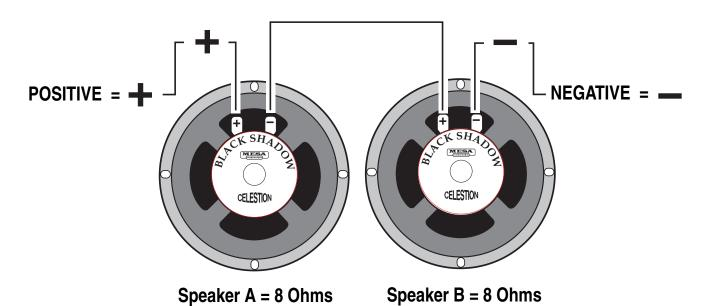
SERIES: Connect the Negative side of Speaker A to the Positive side of Speaker B
