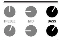
For the most balanced sound and a balance of power between the three rotary tone controls, try to use the TREBLE control in its middle ranges. This scenario produces nearly equal representation of all the frequencies on the tone controls and provides a great neutral starting point for further tweaking.
