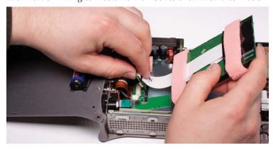
14. While holding down the ribbon cable, slide the small green circuit board piece over the ribbon header mating connector.
