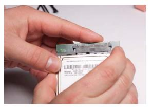
11. With the ribbon face up, attach the two new small nylon screws (included) using a #1 Phillips head screwdriver.
