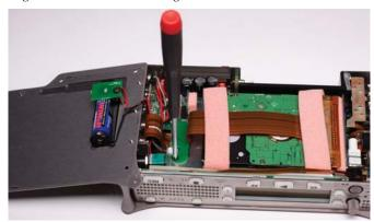
5. Swing the small green circuit board over while pressing down on the ribbon cable to avoid snagging.
