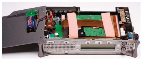
4. Loosen the screw of the small green circuit board holding down the hard drive ribbon cable.
