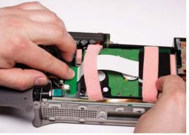
15. Using a #1 Phillips head screwdriver tighten the green circuit board piece securing the ribbon mating connector to the circuit board.
