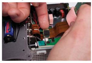
7. Remove the old hard drive and attached ribbon cable from the recorder.
