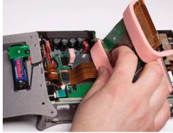
6. Carefully disconnect the ribbon head mating connector from the circuit board.
