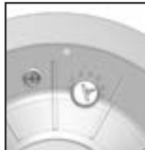
Transformer adjustment from front.
