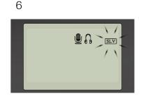
When mode selection is made SLV or MAS icon will blink. (Receive only will not have this option. Skip to step 9)
