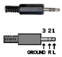
Tip(L or 1 in the illustration) and Sleeve (ground or 3 in the illustration) are wired to the switch if you wish to access port 1 or 3.
