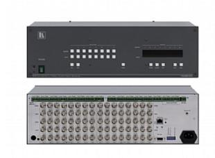
The VS-88HCB is a high-performance universal matrix switcher for composite video, s-video (Y/C) component video (Y, Pb, and Pr), balanced stereo audio and S/PDIF digital audio signals. It can route any or all inputs to any or all outputs simultaneously.
