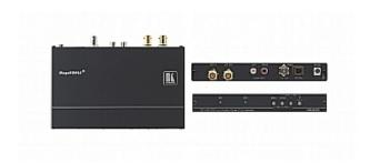
The VP-505 is a high-performance scan converter for SDI, HD-SDI & 3G HD-SDI signals. The unit de-embeds the audio to unbalanced stereo audio & down-scales the video to composite and s-Video (Y/C) simultaneously in either PAL or NTSC formats.
