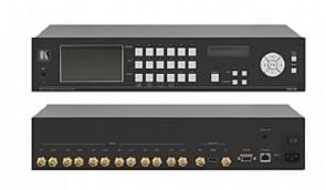
The MV-6 is a versatile, high-performance multiviewer for 3G HD-SDI video signals. The device can display up to six inputs in any combination and output the image in SDI, HDMI and CV formats. Both pre-programmed and customizable screen divisions are supported.
