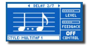
**Advanced** - To enter the advanced menu, press and hold any of the lit BLUE LED soft buttons. To exit the advanced menu, press BACK.
