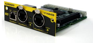
Several signals can be routed to the card for processing and recording, including any bus or Mix Channel (pre or post fade), Input Direct Out, Wedge and IEM monitors, MixRack Inputs, and Input or Mix Insert Sends. Inputs from the card can be routed to Input Channels, Mix External Inputs, Insert Returns, Output sockets and more.
