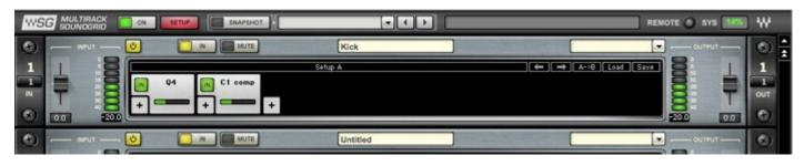
Naming and grouping can be set for each Rack, Plug-in and Rack settings can be stored in Snapshots using the Top bar. Setup design and signal flow can be stored in Sessions. Up to 8 'Hot', important plug-ins can be set for fast access and control.
