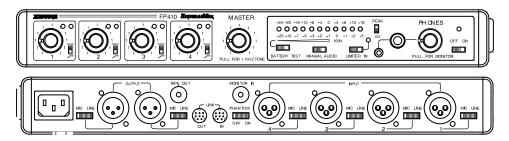
The Shure Model FP410E is an automatic microphone mixer designed for use in a wide variety of multi–microphone speech pickup applications. *Shure IntelliMix* is the remarkable new operational concept behind the FP410E. It delivers flawless automatic mixing by combining three unique functions:
