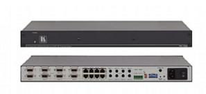
The TP-185 is a twisted pair transmitter for computer graphics, unbalanced stereo audio and RS-232/RS-485 signals. The unit takes up to eight channels of signals and transmits them over eight twisted pair outputs to compatible twisted pair receivers. The TP-185 is also the ideal companion to an eight output matrix switcher – easily converting the outputs to CAT 5.
