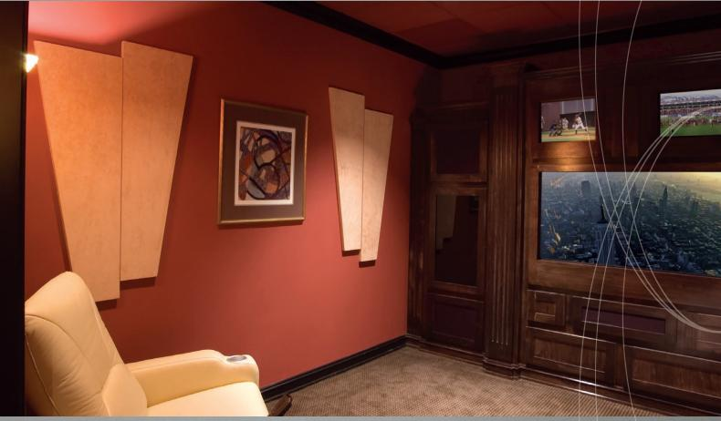
The **SonoSuede HT System** consists of four, 2" thick back-beveled panels predominantly used in the corners of a room to control low frequency anomalies, and eight 1" thick trapezoidal square-edged panels used for taming reflected sound, providing a total of 54 ft<sup>2</sup> of coverage.
