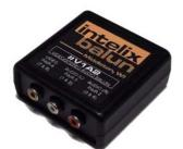
The V1A2 Video Stereo Audio Balun transmits composite baseband video and audio signals via unshielded twisted pair (UTP) cable in a Structured Cabling System. The V1A2 is used in pairs to transmit standard NTSC, SECAM, and PAL composite video. It converts a composite baseband video and 600-ohm stereo audio signal from 75 ohm coax to UTP.
