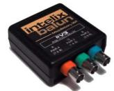
The V3 Balun allows the transmission of composite baseband red/green/blue video via unshielded twisted pair (UTP) cable in a Structured Cabling System. It converts an RGB signal from Coax to three UTP pairs.
