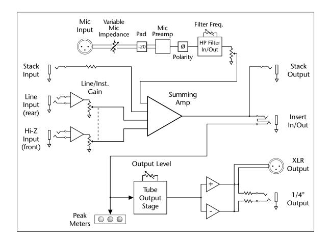
The Impedance control of the 2BA-221 sets the input impedance of the microphone input. The Pad reduces the input level by -20 dB. The microphone input is next amplified by the solid-state preamp before being summed together with the Hi-Z input, line level input and the stacking input. The polarity switch can invert the signal if desired.
