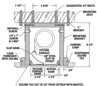
Flush mounting, recessed above ceiling. For use with dropped ceiling. May also be adapted for use with acoustical or other ceiling 1/2" to 3/4" thick but cut to 1/4" thick under doors and screen case.
