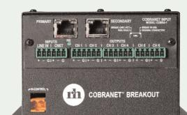
PN series subwoofers can also be connected to a CobraNet Digital Audio Network using the Renkus-Heinz CobraNet Breakout Box shown here.
