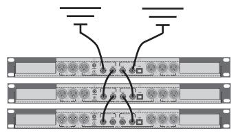
The built-in multi-coupler includes "loop through" outputs for stacking multiple Venue receivers.
