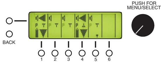
The LCD provides a variety of displays, plus an overview display showing transmitter battery status, RF and audio levels, pilot tone status and diversity switching activity for all six receivers. When receivers are paired for ratio or frequency diversity, the two channels are grouped as such in the overview display.
