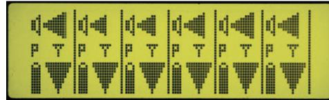
Pressing one of the receiver select buttons under the LCD switches to a detail screen for that module.
