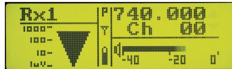
The scanning spectrum analyzer can also be run from the LCD, with manual or automatic location of clear operating frequencies. Scanning can be done with any of the modules to locate clear operating frequencies.
