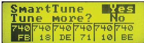
As the receiver is tuned to each frequency, the analysis evaluates RF energy within the channel as well as energy above and below the channel to avoid selecting a frequency adjacent to a high powered signal.
