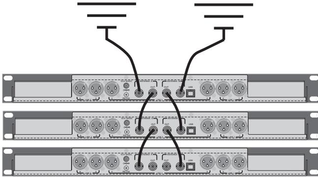
The built-in multi-coupler includes "loop through" outputs for stacking multiple Venue receivers.
