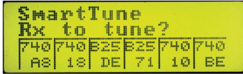
The process takes less than 30 seconds and the screen prompts the operator to turn on a transmitter for the last frequency selected before continuing. Once the transmitter is turned on, the process continues, prompting the operator to continue and select the next receiver to tune.
