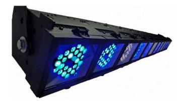
The SPECTRA STRIP is a low profile 6' LED Linear Wash Luminaire with (12) compartments of 50w RGBA Color Mixing or 3000°K high CRI White Light LED Engines. Each compartment can be individually filtered, lensed, or diffused using the dual filter slots provided per compartment.
