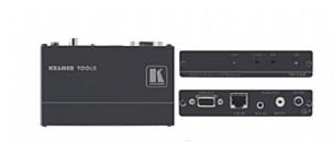
The TP-141 and TP-142 are an extended range twisted pair transmitter and receiver for computer graphics video HDTV) (including and unbalanced stereo audio signals, with high electrical noise immunity. The TP-141 converts computer graphics video and audio inputs to twisted pair signals, and the TP-142 converts the twisted pair signals back into computer graphics video, unbalanced stereo and S/PDIF digital audio signals.
