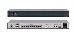
The TP-310A is a high-performance twisted pair receiver and distribution amplifier for computer graphics video, audio and RS-232 signals. The unit takes one twisted pair input and provides ten twisted pair outputs plus two computer graphics video, two stereo audio, two S/PDIF audio and two RS-232 outputs for local monitoring.
