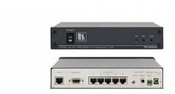
The TP-305A is a high-performance twisted pair receiver for computer graphics video, audio and RS-232 signals. The unit takes one twisted pair input and provides five twisted pair outputs plus a computer graphics video, stereo audio, S/PDIF audio and RS-232 output for local monitoring.
