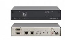
The TP-200AXR is a twisted pair receiver for computer graphics video and unbalanced stereo signals. The TP-100AXR converts the input signals into a twisted pair signal and the TP-200AXR converts the twisted pair signal back into two computer graphics signals, as well as two stereo audio plus two S/PDIF audio signals.
