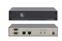
The TP-100AXR is a twisted pair transmitter for computer graphics video and unbalanced stereo signals. The TP-100AXR converts the input signals into a twisted pair signal and the TP-200AXR converts the twisted pair signal back into two computer graphics signals, as well as two stereo audio plus two S/PDIF audio signal.
