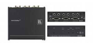
The VP-2K is a highperformance distribution amplifier computer for graphics video signals, with resolutions up to and exceeding UXGA, and unbalanced stereo audio signals. The unit distributes one input signal to two identical outputs.
