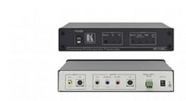
The FC-10Dxl is a high-performance bidirectional transcoder for composite and s-Video (Y/C) signals. The unit converts a composite video or s-Video input through a digital comb filter to a composite and s-Video (Y/C) or component (YUV/RGB) video output.
