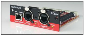
The M-DANTE option module is one of a range of option cards. It gives access to 64 input and 64 output channels and can be fitted to the Port B expansion slot in iLive fixed format MixRacks (iDR-16, iDR-32, iDR-48 & iDR-64) or expander (xDR-16). It can also be fitted to iLive modular MixRacks (iDR-0, iDR-10), and Port A of iLive surfaces 80/112/144/176 if they are fitted with the new RAB-2 standard with appropriate firmware version installed (1.71 or higher).
