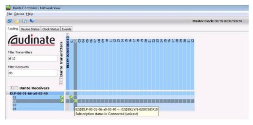
Clicking matrix crosspoints in the Routing page allows transmitting audio channels from the iLive system to any other device in the network, as well as receiving channels.
