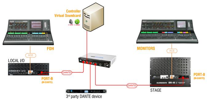
The iDR-48 Monitor system is the clock master for the network. The iDR-16 is the FOH system receiving most of its inputs digitally via Dante. The main outputs from the iDR-16 are also sent to a Dante-enabled loudspeaker processor or amplifier. A desktop computer is being used to control the DANTE network and record all audio signals sent from the iDR-48.
