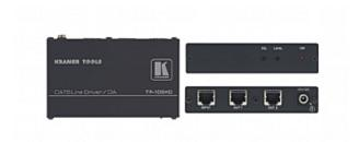
The TP-105HD is a line driver and distribution amplifier for analog video over twisted pair signals. It takes a twisted pair input and distributes it to two identical twisted pair outputs.
