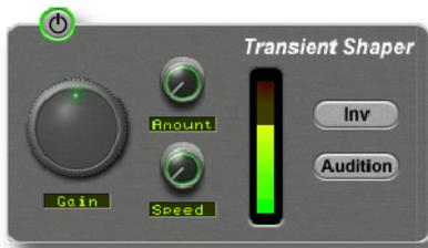
The Transient Shaper allows you to add attack to the start of a drum hit by increasing the amplitude of the attack portion of the signal whilst leaving the decay unchanged. The right hand waveform is a processed version of the one on the left. It has been passed through the transient shaper where the amplitude of the attack portion has been increased.
