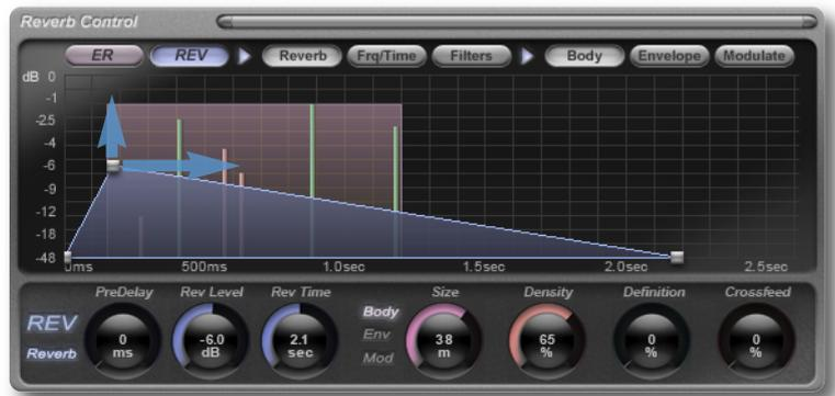
When **Freq/Time** or **Filters** is selected, the graph changes to display the Frequency/Time blocks and High/Low Shelving filter curves. Both graphs are overlaid with the active graph being in focus (on top).
