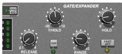
To activate the Expander/Gate, turn the **RANGE** knob so that it’s range is no longer zero. The green indicators in the right-hand of the two meters in the centre of the Dynamics section show the amount of gain reduction being introduced.
