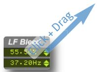
The frequencies and slope of the bleed-band filters are indicated either side of the graph; LF to the left and HF to the right. The slope is measured in percentage.
