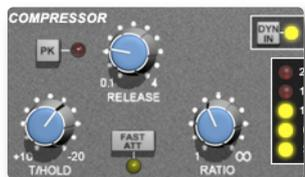
To activate the Compressor/Limiter, turn the **RATIO** knob so that it’s ratio is no longer 1:1.
