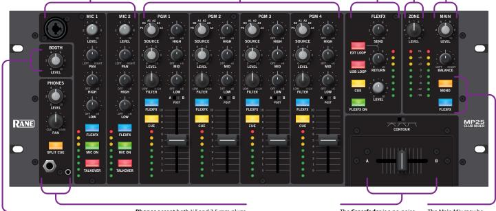
The **Booth** Output includes a Level control and auto-mono balanced 1/4" TRS outputs.
