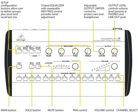
selects the MAIN stereo bus SOLO button allows user to listen to selected inputs
