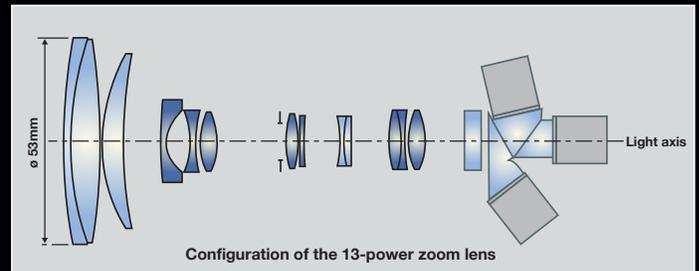
The wide-angle zoom lens that gained high popularity in the HVX200 Series has been reduced in size, lightened, and further widened in this 13x zoom lens. The lens structure combines 13 lens elements in 10 groups, with 3 aspherical lenses. The diameter of the front lens element has been reduced from 67 to 53.2 mm, while still achieving a 28mm wide angle (35mm equivalent), the widest of the class.\*
