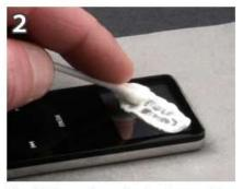
A soft-tipped applicator is used to polish across deep scratches and blemishes - use moderate to light polishing pressure.
