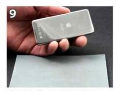
Check surface periodically to avoid abrading through the chrome plating. If any faint tan color is noticed-STOP. Repeat steps 1-3 to complete the final finish.
