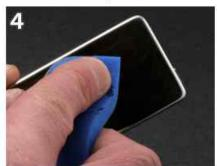
Using a section of blue refinishing pad, rub rough side across individual scratches and blemishes. Once all major defects have been knocked-down, proceed to step 5.
