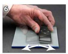
Slightly rotate convex and rounded surfaces to evenly refinish.
