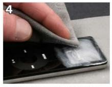
Fold an Optex cloth in fourths. Polish using circular motions, light to moderate pressure - don't press so hard as to push through the compound. Let it do the work.
