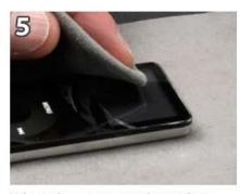
When the compound vanishes, check the surface and reapply A compound as needed - each application progressively removes more damage. Repeat until all major defects are gone.
