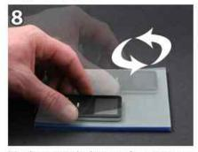
Moderate to light circular motions across pad will produce a non-directional bright finish. Continued light cycle polishing will produce a mirror-like finish.
