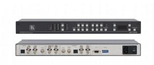
The SP-12HD is a broadcast quality video processor that functions as a ProcAmp, TBC and format converter for composite video, s-Video (Y/C), component video (YUV) and HD-SDI video signals. The original and processed images can be viewed simultaneously with the split screen output enabled.
