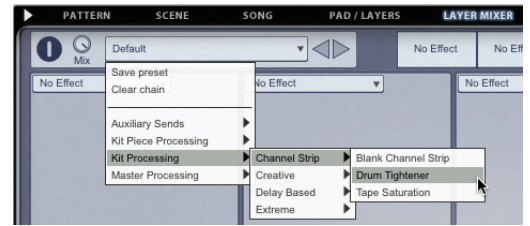
Using the Chain picker to select a preset for the entire FX chain.
