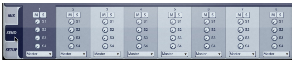
When Sends view is active, Send 1-4 controls for the 4 Aux busses are shown with the Mute , Solo and Output selector .
