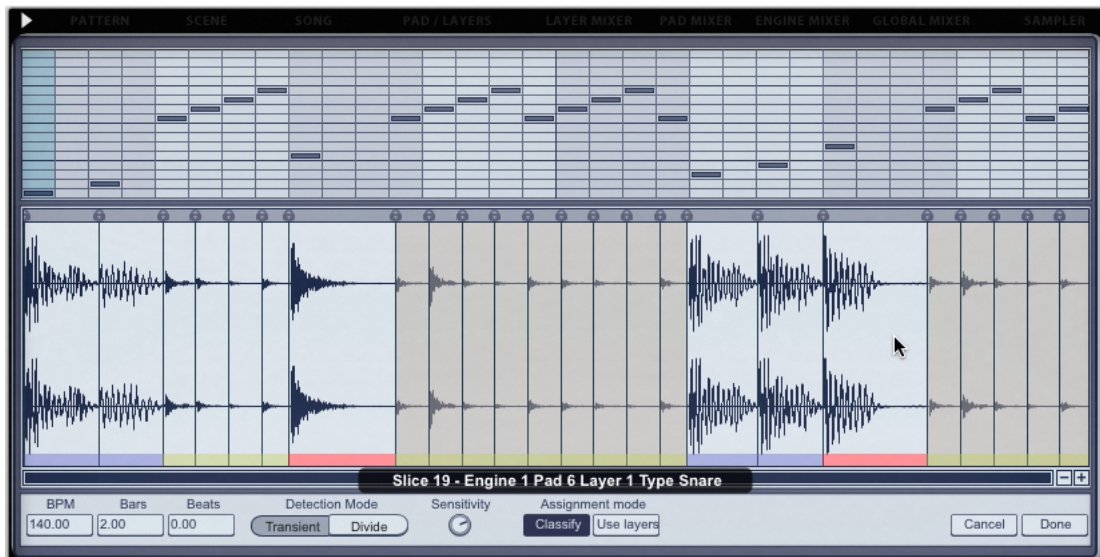
Extracted slices are highlighted more brightly than unused slices. The coloured strips below the waveform indicate the slice's classify status. Hover the mouse over a used slice to show information about the pad/layer to which the slice has been extracted.
