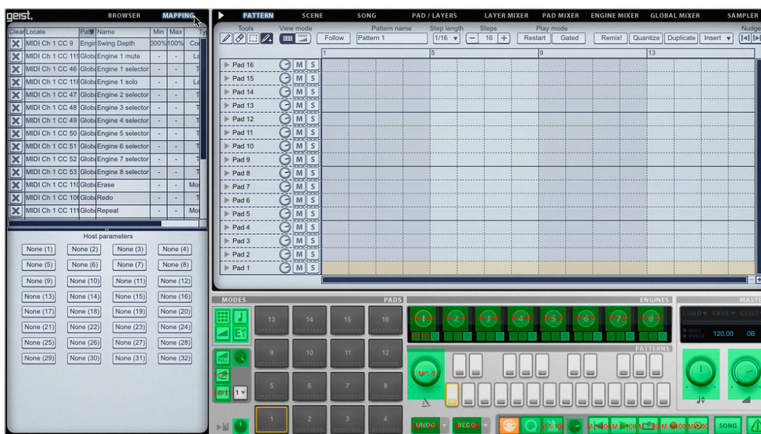
This screenshot shows the Mapping panel after some MIDI CC assignments have been made.
