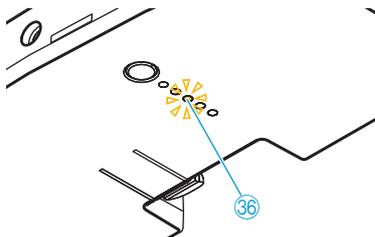
The charge status indicator 36 goes off after approx. 5 seconds. The LED 3 then display the status of the charging electronics.
