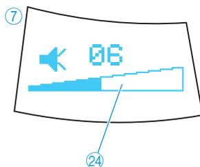
The loudspeaker volume is changed. The multi-function display **7** shows the volume of the conference units' loudspeakers **24**.
