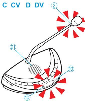
When the chairman assigns you the “speaking right”, your microphone switches on. The microphone LED ⑩ and the signal light ring ② light up red. The loudspeaker ⑳ is muted. Depending on the conference mode and the speaker limit set, the microphone of the previous speaker will be switched off.
