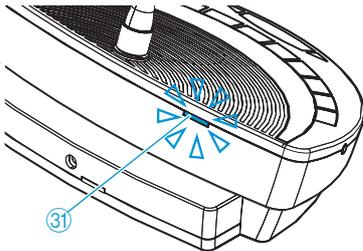
When the battery pack is almost flat, the status indicator 31 indicates the remaining operating time.
