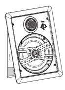
**8** Tighten each of the four screws evenly until the clamps at the back of the frame grip the wall to secure the speaker.
