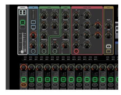
The Virtual Si Compact features an additional 'CONTROL' zone; this replicates the fader, ON and SOLO keys of the currently selected channel or bus.
