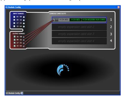
The names of the card (in green) can be edited to help give meaning to the card or application. These names will then be used on the console touch screen.
