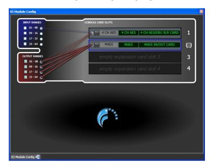
To configure the stagebox 'right click' on any slot to remove a card or add a card. For help in understanding the various configurations click on the '?' icon to open a browser and download copy of the <u>Soundcraft Studer I/O Racks manual</u> which describes the rules that govern legal card configurations.
