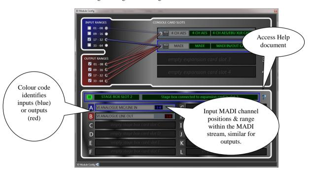
This configuration shows both cards receiving signals from all channels of the Si expansion bus, but the AES card is routed to expansion bus inputs 1-8 whilst the MADI card is routed to inputs 17 to 64.
