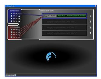
**NOTE**: When a card is added, the system will by default set all OUTPUT routing switches 'ON'.
