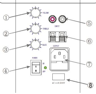
■ Features: 30 Watts rms - Audience Size 500, Room size 1,000 sq.ft. ■ 5" Full Range Speaker (8 Ohms) 1" Dome Tweeter ■ One Stereo RCA Input & Stereo Speaker Terminals - INCLUDES 10 Ft. Cable to connect auxiliary speaker ■ Treble and Bass Controls ■ AC Power cord Specially tooled and molded plastic enclosure for exceptional durability Weight 10 lbs.
