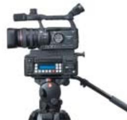
Connect Ki Pro to a wide variety of professional HD cameras via component or HD-SDI. The Apple ProRes 422 recordings that Ki Pro produces rival the native recordings of many HD cameras. Apple ProRes 422 recordings are full raster video at 10-bit quality whereas typical camera recordings produce a variety of compressions, horizontal resolutions, file types, and are often only at 8-bit.
