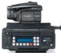
Connect prosumer HDV and AVCHD camcorders via HDMI to Ki Pro. Ki Pro enables cost-effective cameras to produce professional quality recordings in Apple ProRes 422 and Apple ProRes 422 (HQ).
