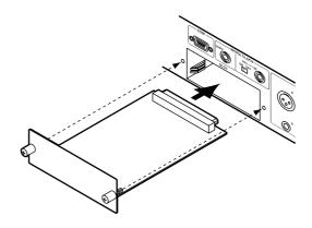
4 Secure the card using the attached thumbscrews. Do not leave the thumbscrews loose, as the card will not be grounded correctly.
