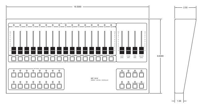
The MC 1616 control console delivers complete flexibility in entertainment lighting applications with 16 individual control channels and 16 pattern memory buttons. Any of 16 memories are programmable for chase effects or static scenes. The advance rate of individual pattern steps is selected by a chase tap control or may be synchronized to audio via an audio line input port.
