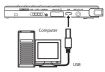
If you connect the unit by USB when its power is ON, or if you turn the unit's power ON when it is already connected by USB, a screen appears on this unit's display to let you choose whether you want to operate the unit using USB bus power or to connect the unit with the computer by USB.
