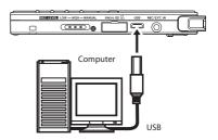
When connected to a computer, a pop-up window appears on this unit's display to let you choose whether you want to operate the unit using USB bus power or to connect the unit with the computer by USB.
