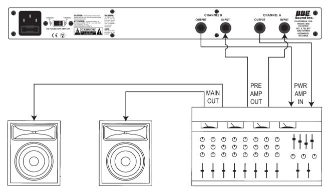
Option 2: Connect using individual channel or main insert points.
