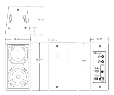
UMH (Universal Mounting Hardware) attachment points are standard on all fixed installation models. The points have Metric M6 threads and are positioned 1 3/4" from the edges unless otherwise indicated. A nut-plate for Omnimount Series 60 mounting hardware may be substituted for the UMH points; can be either top, bottom or side mounted. U-bracket attachment points are a third option.
