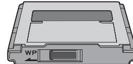
Only change the write protect switch position before inserting the card into Qio
