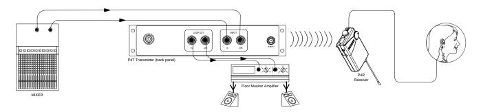
**Operating Floor Monitors Through a P4T Transmitter:** Send an audio signal through the LOOP connectors to a floor monitor amplifier. In this set up, the receiver and the onstage monitors reproduce the same audio.
