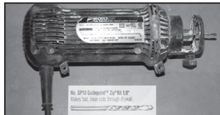
Fig. 11: Rotozip™ showing guidepoint bit.
