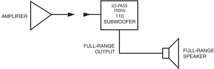
PASSIVE 110 INPUT MODULE—LO PASS FILTER
